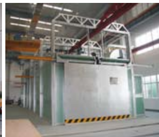
The VTS200 is epoxy painted and temperature cured eliminate corrosion
