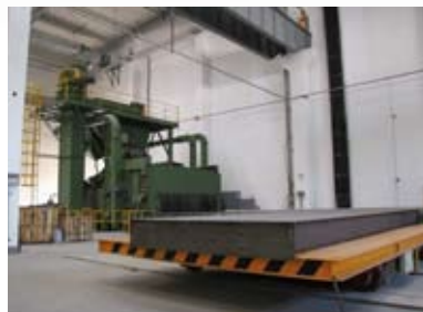
The steel in the VTS200 is shot blasted to create a fantastic painting surface
